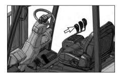
Move the directional control forward/reverse switch to NEUTRAL.
