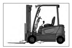
7. Block the wheels if parking on an incline.
