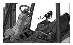
To slow, stop or change direction when traveling in either direction, move the directional control lever (1) to the opposite direction while keeping the accelerator pedal (2) depressed.
