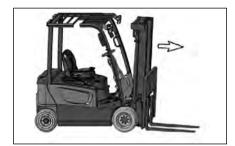
1. Tilt the mast to the full forward position.
