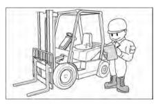
Inspect and check the condition of your forklift truck using the operator's check list before starting work. Immediately report to your supervisor any obvious defects or required repairs.
