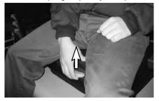
Pulling the weight adjusting lever upward, move it right or left to adjust the weight input based on your weight (50–130 kg).
