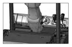
16. Adjust the steering wheel to comfortable position. Grasp the steering wheel and raise the handle to release the steering column. PULL the steering column BACK or PUSH FORWARD to obtain the most comfortable position. RELEASE the knob and make sure the steering column is locked in this position.
