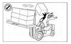
Do not operate your truck without the load backrest extension and overhead guard. Keep the load against the backrest with the mast tilted backward.
