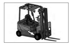
Inspect the drive axle housing and the ground for oil leaks. Refer to "Drive Axle" in "When Required" section, if an oil leak is found.
