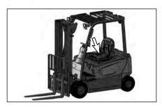
the seat switch is located under the operator's seat.
