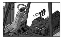
Move the directional control lever to the opposite direction of lift truck travel.
