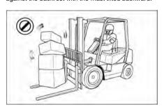
Do not lift or move loads that are not safe. Do not pick up an off center load. Such a load increases the possibility of a tipover to the side. Make sure loads are correctly stacked and positioned across both forks. Always use the proper size pallet. Position the forks as wide as possible under the load. Position loads evenly on the forks for proper balance. Do not lift a load with one fork.
