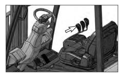
Move the directional control forward/reverse switch into the NEUTRAL position, if it is not already in this position.
