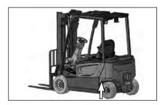
2. Remove the hydraulic tank drain plug. Allow the oil to drain. Clean and install the plug.
