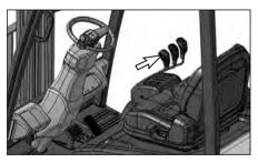
Move the directional control forward/reverse switch into NEUTRAL.
