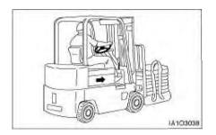
Carry the load as low as possible, while still maintaining ground clearance.
