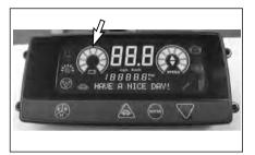
A fully charged battery will cause a "9 segments" to be displayed on the LCD display. As the battery is discharged, the LCD display will count down, 9, 8, 7, and etc., until "EL" is displayed. When the battery reaches 80% discharge level, the Micro-Controller will cause the LCD display to continuously index through the entire range (1 through 9 segments) to signal that the battery is discharged and lift interrupt is imminent
