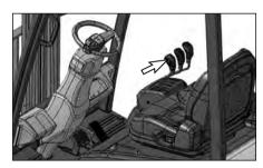
Move the directional control forward/reverse switch to the direction of travel.
