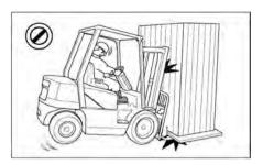
Do not overload. Always handle loads within the rated capacity shown on the capacity plate.
