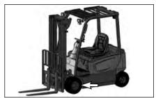
6. Inspect the tires, valve stems and wheels for cuts, gouges, foreign objects and loose or missing nuts. Refer to "Tires and Wheels" in "Every 10 Service Hours or Daily" section, if repairs or replacement is necessary.
