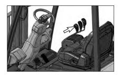
Check the tightness of the directional forward/reverse switch mounting bracket. Adjust if needed.
