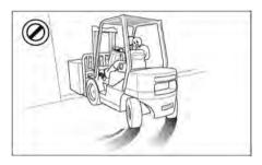
Do not start, stop, turn or change direction suddenly or at high speed. Sudden movement can cause the lift truck to tip over. Slow the speed of your truck and use the horn near corners, exits, entrances, and near people.
