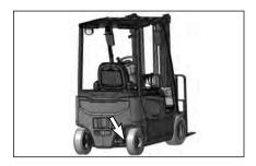
Lubricate fitting on steer axle.
