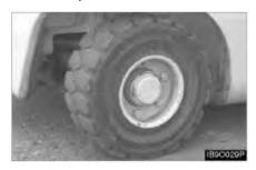
Install the steer wheel. Put two nuts opposite each other (180°). Tighten both. Install all remaining nuts. Tighten all nuts in a crisscross sequence opposite each other (180°) to a torque of 140 N·m (105 lb-ft).
