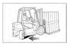
Do not drive in forward direction when loads restrict your visibility. Operate your lift truck in reverse to improve visibility except when moving up a ramp.
