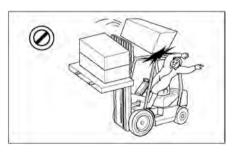
Do not move loose loads that are higher than the load backrest.
