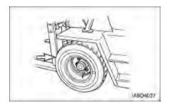
Check all components carefully and replace any cracked, badly worn, damaged and severely rusted or corroded parts with new parts of the same size and type. If there is any doubt, replace with new parts. Do not, under any circumstances, attempt to rework, weld, heat or braze any rim components.
