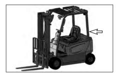
Inspect the overhead guard for damage, loose or missing mounting bolts.
