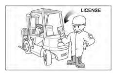
Only properly trained and authorized personnel should operate forklift trucks. Wear a hard hat and safety shoes when operating a lift truck. Do not wear loose clothing.
